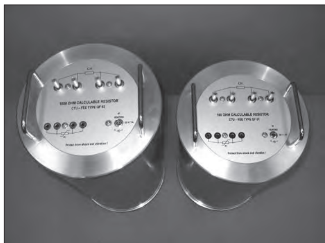
Obr. 2.9.7: Etalony QF01 (100 Ω) a QF02 (1 000 Ω)
